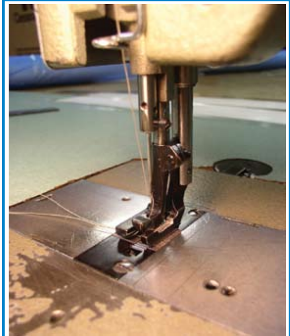
The business end of a walking foot needle feed machine. All this stuff moves with the material being sewn.
