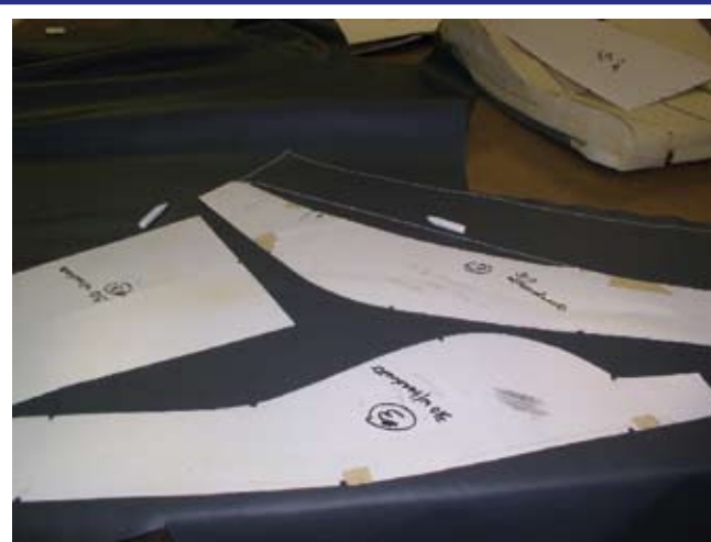
Efficiently laying out patterns on the raw material.
